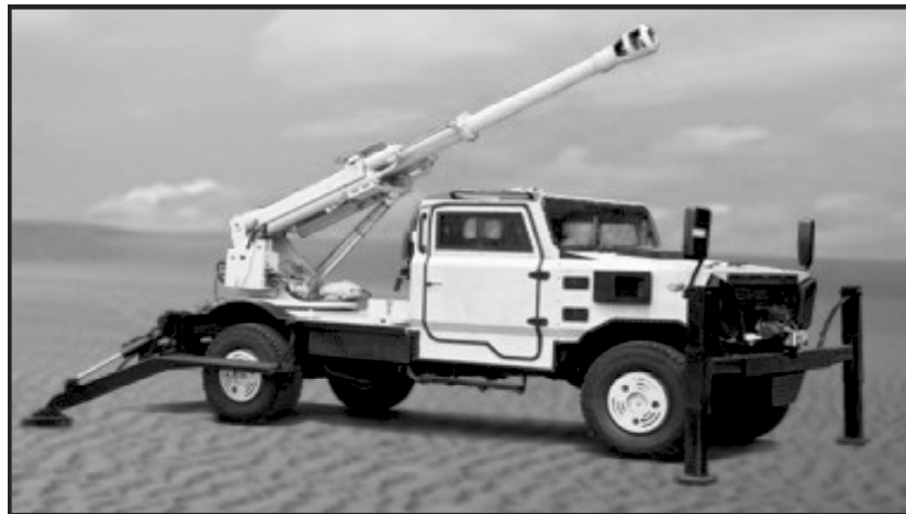
Image 3: Garuda 105/37 mm system (Lightweight Trails and Platform Stabilisers)
